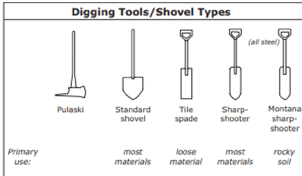
Figure 10. Shovel styles and primary uses, from the NRCS Field Book for Describing and Sampling Soils (Schoenberger et al. 2012, section 8-5). Typically, a sharpshooter style is best for digging soil pits because of its narrow profile, which results in less surface damage than a standard shovel.
