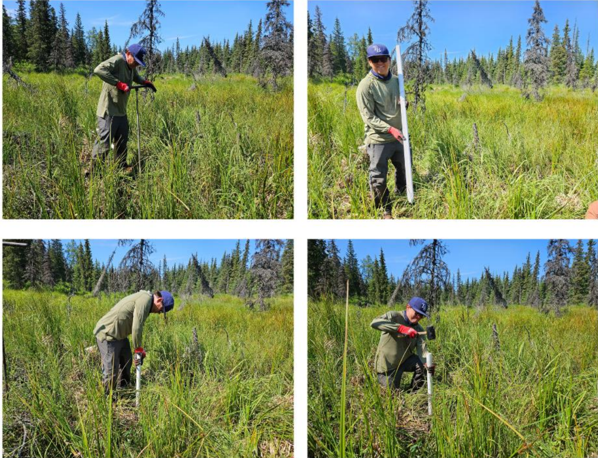
Figure 12. Steps for installing a simple, shallow water-table well in a peatland to measure changes in water level. Photo credit: USF-ERG.
