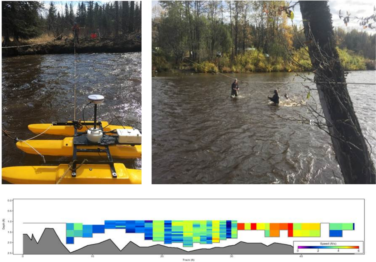
Figure 2. The Acoustic Doppler Profiler (SonTek) allowed us to measure stream discharge during high flow events. Prior to the use of the SonTek, sampling discharge high water events required ropes and taller staff members (above right). A graphical output from the profiler illustrates a rough outline of the river bottom and colored cells representing water speed in feet per second (below).
